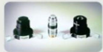
Darkfield attachment Imm. DF Condenser with OBJ 100x having Iris Diaphragm Dry. DF condenser
